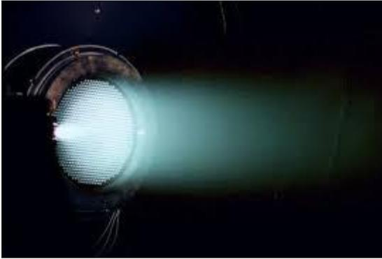
Ion engines are more sensitive to the chemical properties of the fuel. In them, the atoms of the working fluid receive an electric charge and are accelerated in an electric field. Oxygen or nitrogen oxides are dangerous for ion engines and can burn electrodes. But ion engines can run on nitrogen.
