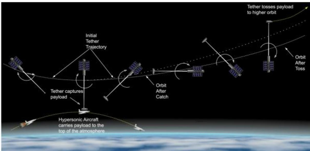
The speed at the end of the rotating cable can be either less or more than the speed of the sling itself, depending on the position in space. For example, the sling can pick up cargo from the "Suborbital flight", having a speed below the space. After that, the load, climbing the cable, can accelerate to orbital speed.
